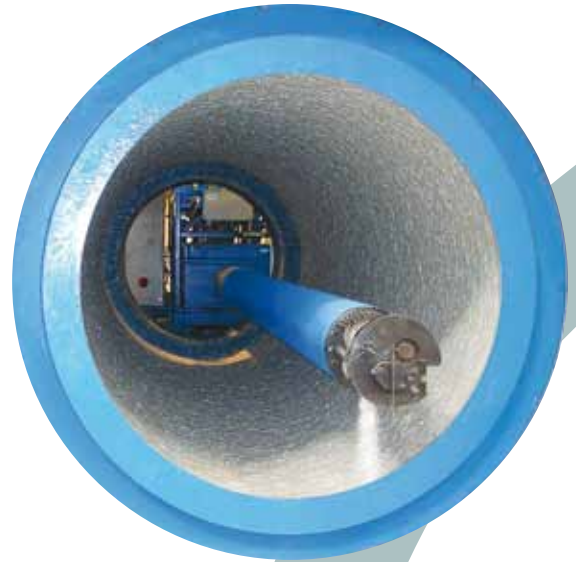
Centrifugal casting process patented by HOBAS
